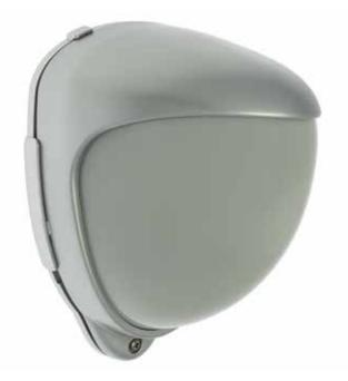
The DET-REXT-PIR30 is an outside radio detector for perimeter protection. The unit uses two independent, different technology detectors, both of which must trigger to cause the detector to signal an alarm. The detector delivers precise, reliable presence detection. Combining Scantronic's class leading radio with GJD's reputation for flexibility, stability and accuracy to identify a threat before they have a chance to cause loss or damage.
