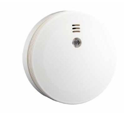
Providing a flexible solution to smoke detection, it has its own built-in sounder for local alarms and can be programmed to trigger control panel sounders.
