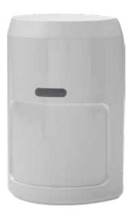
A wired passive infrared movement detector with dual low noise sensor and excellent RF immunity. The DET-WPIR-00 offers a detection range of 15m and is also equipped with adaptive temperature compensation.
