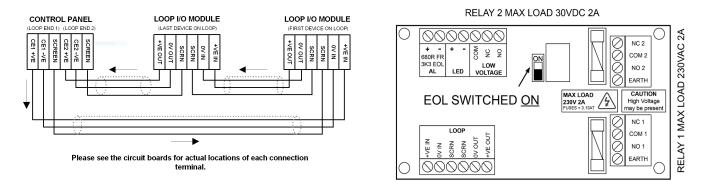
Before installing the module remember to note the serial number of the device (located on the rear of the unit) on to your drawings or configuration sheets to enable you to prove its location later. The address allocation for the device is carried out automatically by the control panel whilst in initialisation mode, so addresses do not need to be set manually.
