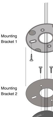
2. Screws the Mounting Bracket as below diagram.
