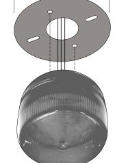
3. Spin the Mounting Bracket 2 and strobe light unit to lock on ceiling.
